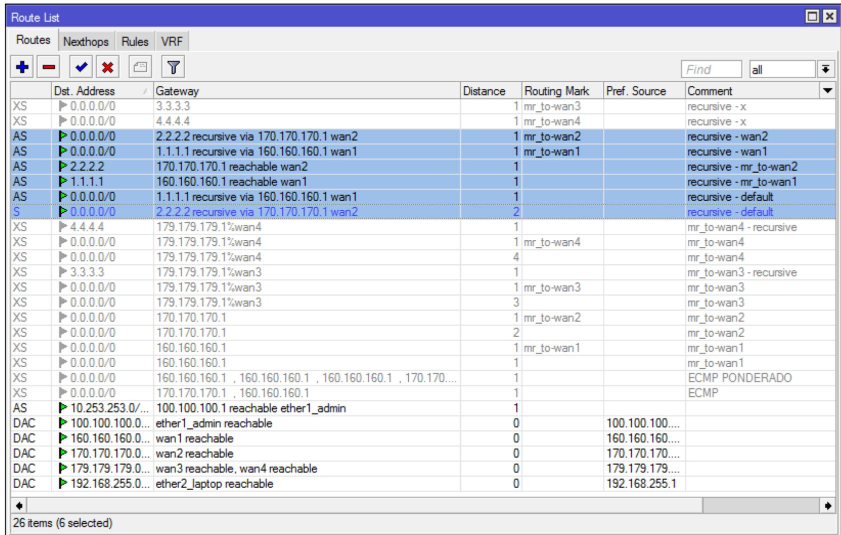
The screenshot shows a 'Route List' window with a table of network routes. The table has the following columns: Dst. Address, Gateway, Distance, Routing Mark, Pref. Source, and Comment. The routes are listed in descending order of preference. The selected route is highlighted in blue.
