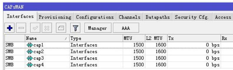
The screenshot shows the CAPsMAN configuration interface, specifically the 'Interfaces' tab. It displays a table of configured interfaces. The table has columns for Name, Type, MTU, L2 MTU, Tx, and Rx. Four interfaces named cap1, cap2, cap3, and cap4 are listed, all of type 'Interfaces' with an MTU of 1500 and L2 MTU of 1600. The Tx and Rx rates are both 0 bps.
