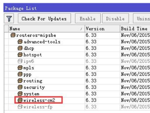
A screenshot of the Mikrotik Package List interface for a CAP access point. The interface shows a table of installed packages. The 'wireless-cm2' package is highlighted with a red box. The table has columns for Name, Version, and Build Time.
