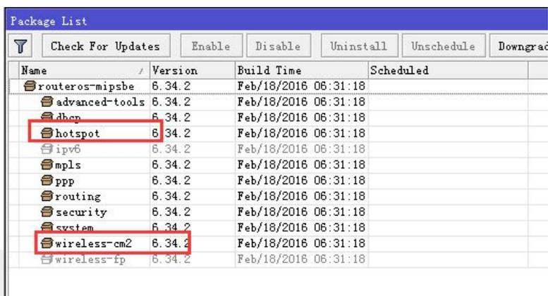
A screenshot of the Mikrotik Package List interface for a CAPsMAN control plane. The interface shows a table of installed packages. The 'hotspot' and 'wireless-cm2' packages are highlighted with red boxes. The table has columns for Name, Version, Build Time, and Scheduled.
