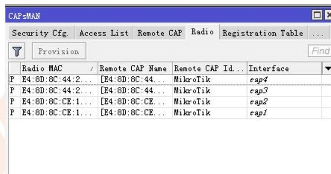
The screenshot shows the CAPsMAN configuration interface, specifically the 'Radio' tab. It displays a table of radio connections. The table has columns for Radio MAC, Remote CAP Name, Remote CAP Id..., and Interface. Four entries are listed, each with a MikroTik remote CAP name and a corresponding interface (cap4, cap3, cap2, cap1).
