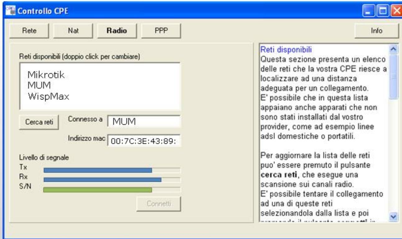
The application shows in real time the signal/noise level and the tx/rx quality for the connection. It allows to find the base station and to point the antenna also without technical experience.
