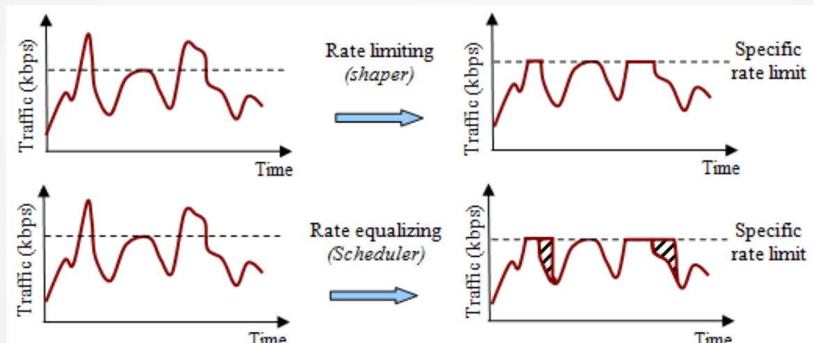
Figure 8.1. Principles of rate limiting and equalizing
