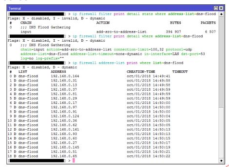
/ip firewall filter will not PROCESSed some rule if the PACKET already caught in /ip firewall raw and for some example is:
