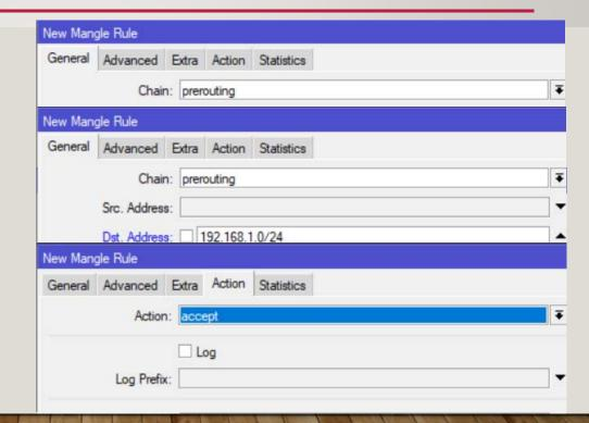
Add PCC (Per connection Classifier) Rules to SORT the traffic into STREAMS
