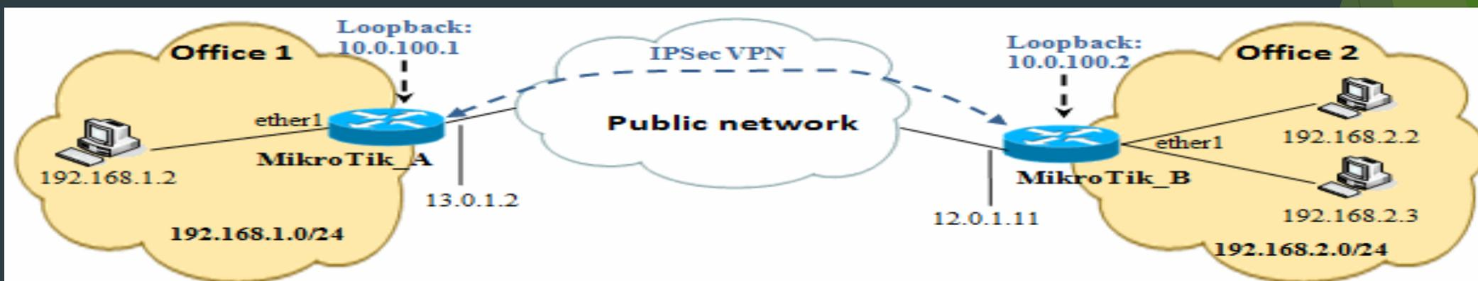
Figure 9.11. Network example with IPSec VPN
