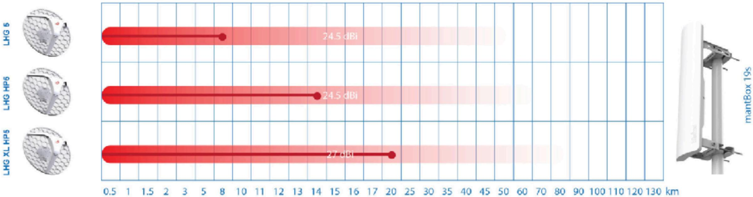
○ Distance at max supported 802.11a data rate (eg. 865Mbit/s) ● Distance at max supported 802.11n data rate (eg. 300Mbit/s) ■ Max range at -70dBm signal
