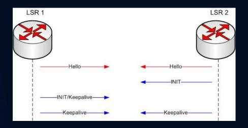
Label Distribution Protocol (LDP) — Similar to a routing protocol, LDP maintains the database of MPLS labels and exchanges labels with other LDP neighbors. LDP relies on the underlying routing information provided by an IGP (OSPF, IS-IS, EIGRP) in order to forward label packets. MPLS Forwarding – Routing FIB vs. MPLS FIB (or LFIB)
