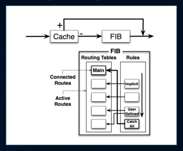
MikroTik Routing Forwarding Information Base (FIB) — When a Non-MPLS routed network needs to forward a packet, it does so via the FIB which is usually a mirror of the routing table.
