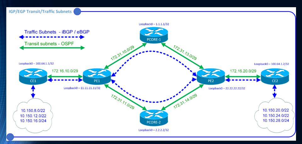
BGP/OSPF — OSPF builds the topology of the network and provides loopback and next hop reachability for BGP and MPLS. BGP then utilizes MPLS to advertise customer VRF subnets and maintain logically separate routing tables in the VPNv4 community.
