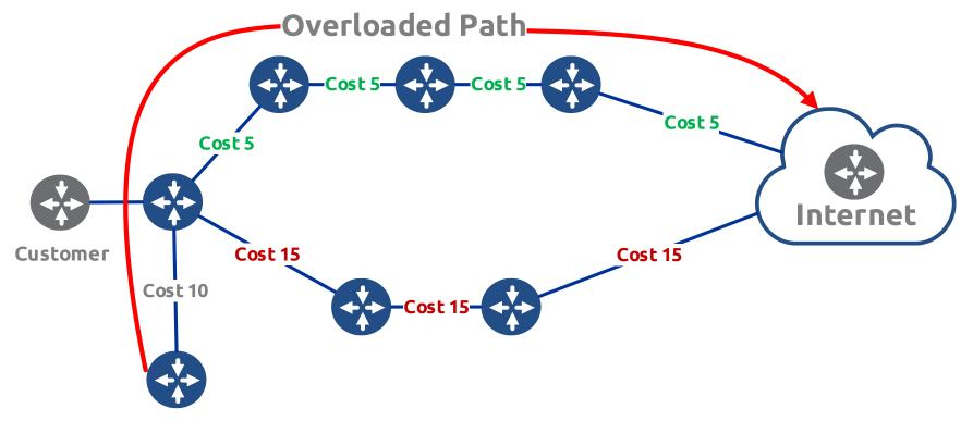
**Example:** With the addition of the new tower, we need to utilize bandwidth down both paths.
