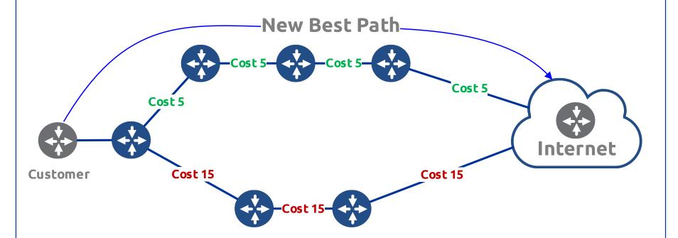
**Example:** Cost has now been modified to 5 on each link for the faster path and 15 on each link for the slower path.
