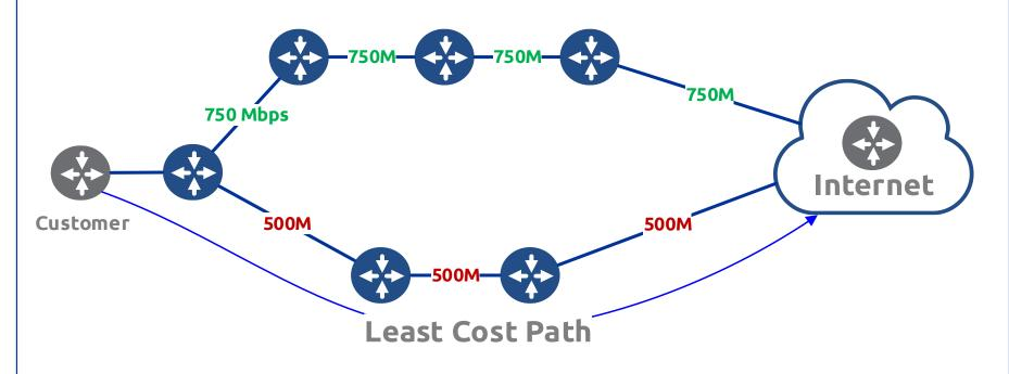
**Example:** OSPF when using default Gigabit cost (10) will select the "shortest" path – but not the fastest.
