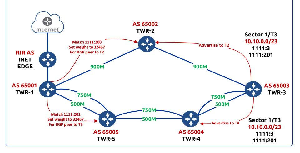
**Influencing traffic down one path:** By tagging the subnet for Sector 1 at Tower 3 (10.10.0.0/23) into community 1111:201, we are able to force the traffic along the higher capacity but less preferred southern tower path.
