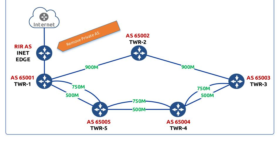
**Combining OSPF TF and eBGP:** In order to build an eBGP design but still leverage the OSPF TF for capacity, we have to build a multihop eBGP peering using the OSPF TF loopbacks in blue. Then the BGP loopbacks in red can be advertised as the reachable loopback outside of that router.
