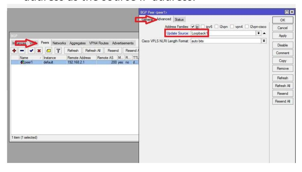
Make sure each router has IP routes so that they can forward packets to the loopback interface IP address of the other router.
