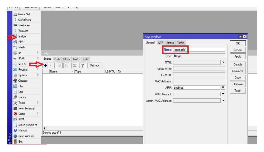
**Step 2**Configure an IP address on a loopback interface on each router.
